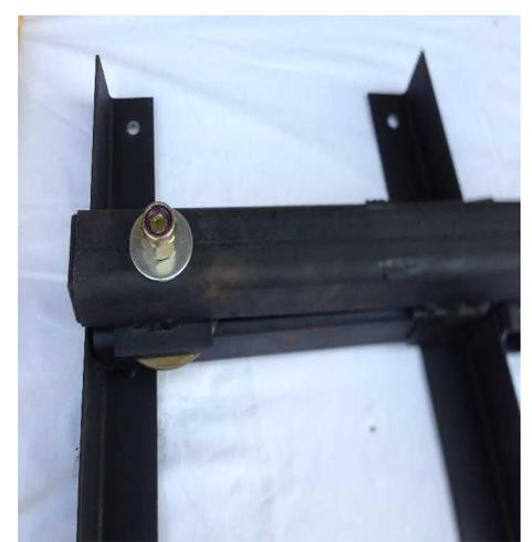
Flip both pieces over and use N & P to tighten the bolt. Tighten it enough so where there is no slack but loose enough it will still rotate.
