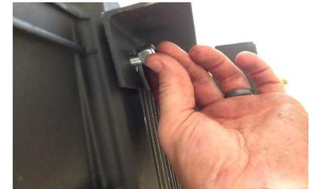
Push the C's up through the bottom if you want to force the box to be open to remove the nuts (more secure). Screw B's onto C's. Do not over tighten to the point the floor deforms. Installation complete.
