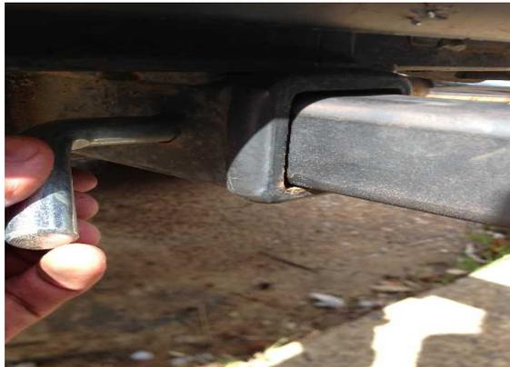
Insert the entire assembly into the receiver of your vehicle and secure with I & J.
