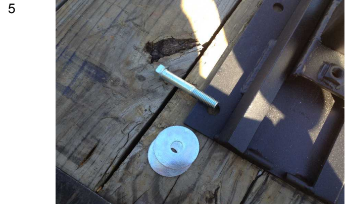
Place the ATV in the trailer and position where desired then arrange the unit underneath the ATV in a place that will allow it to connect to the ATV with some room for adjustment. Make sure at least 2 of the bolt holes will be positioned to go through the steel cross members under the trailer. Use one J through the top of each hole in A & two B's with one I underneath the trailer floor.
