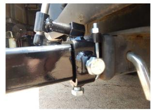
Push C up against truck receiver then tighten nuts. (Do not over tighten). Push E up against C then tighten bolt on side first then the bolt on bottom.
