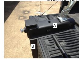
ATTACH (A) TO ATV HITCH BY MOVING IT DOWN (B) & TIGHTEN SET SCREW. NOTE: ONCE SET TO YOUR ATV DO NOT REMOVE SET SCREW.
