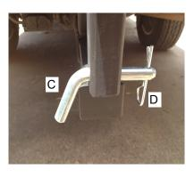
TO UNLOAD ATV, REMOVE COTTER PIN(D) & CLEVIS(C), LOOSEN SLIP HANDLE(F), & LIFT (B) OUT OF (E).
