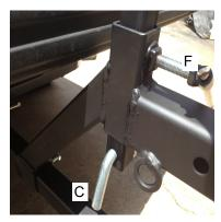
INSERT (B) INTO (E) & INSTALL (C),(D), & (F) DO NOT TIGHTEN (F).
