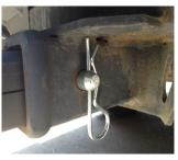
ALIGN HOLES IN (G) WITH HOLES IN TRUCK RECEIVER THEN INSTALL CLEVIS & COTTER PIN ENSURE COTTER PIN IS SECURED PROPERLY.
