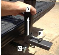
RAISE (B) UP UNTIL IT STOPS AGAINST (C) THEN LIGHTLY TIGHTEN (F) TO HOLD
